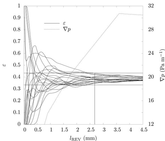
**Fig. 2.** Solid lines: porosity for growing cubic volumes around 20 random points for the wet snow sample. The two horizontal lines indicate the tolerance bandwidth  $\xi = 0.05$ . The vertical line indicates the chosen REV length. Dashed line: pressure drop for growing vertical length of the wet snow sample.
