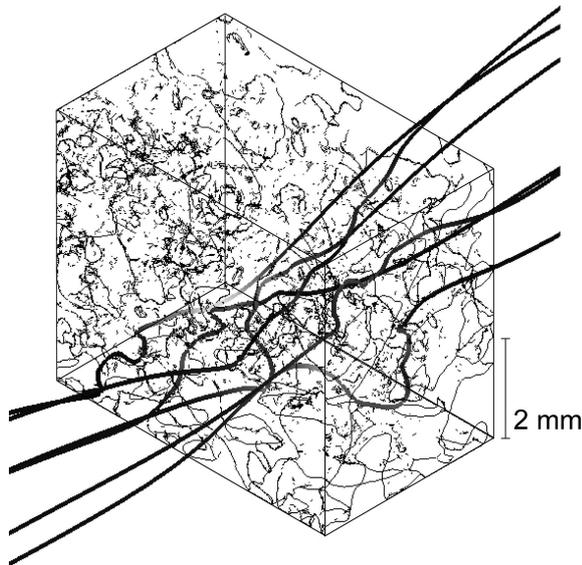
**Fig. 1.** 3-D surface rendering of the wet snow sample (ws, as listed in Table 1) with fluid flow streamlines.
