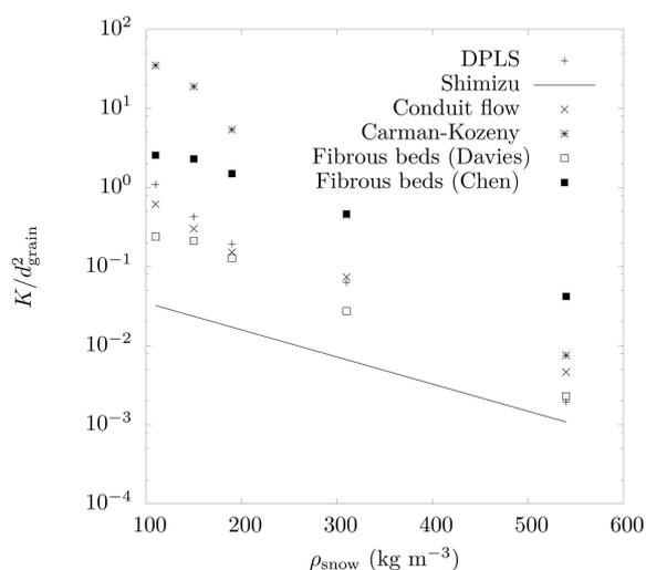
**Fig. 6.** Permeability (dimensionless,  $K/d_{\text{grain}}^2$ ) as a function of snow density for CT-based DPLS and for theoretical and empirical models.
