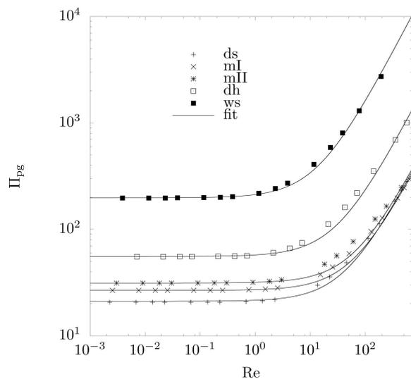
**Fig. 4.** Calculated (symbols) and fitted (curves) dimensionless pressure gradient as a function of  $Re$  for the five characteristic snow samples (see Table 1).
