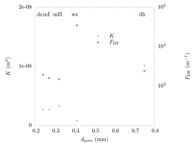
**Fig. 5.** Permeability and Dupuit-Forchheimer coefficient versus pore diameter.
