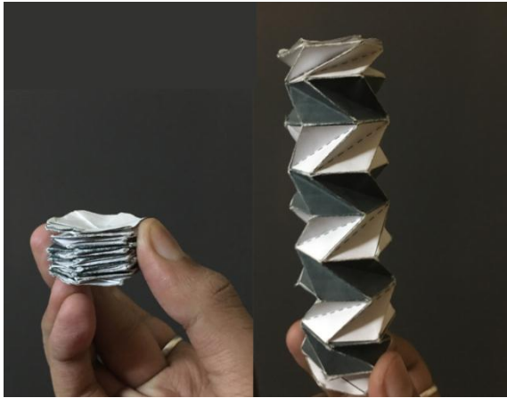
Figure 2- Kresling patterned bellow in contracted and expanded position.
