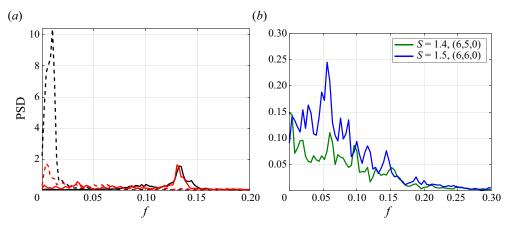
Figure 13. Power spectral density estimate for the time series of (a) fluctuating velocity components for bubble form of vortex breakdown (BVB),  $u'_x$  (----) and  $u'_y$  (-----) obtained on the axis (y = z = 0) at x = 8 at S = 1.3 (black) and x = 6 for S = 1.4 (red) and (b)  $u'_y$  for conical form of vortex breakdown (CVB) at different S and (x, y, z) probe locations.
