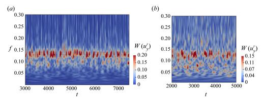
Figure 14. Scalogram showing the magnitude of the continuous wavelet transform of  $u'_y$  for x = 8 on the axis for the bubble form of vortex breakdown at (a) S = 1.3 and (b) S = 1.4.
