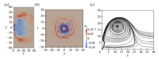
Figure 22. Flow features for case S = 2.15 and Re = 1000 simulated in a larger domain of  $L_y = L_z = 80$  and  $L_x = 40$ : instantaneous axial velocity contours on (a) z = 0 and (b) x = 2 planes, and (c) time-averaged features shown using projected streamlines based on mean velocity field. The axial velocity range shown is chosen for clarity and is smaller than the actual range.
