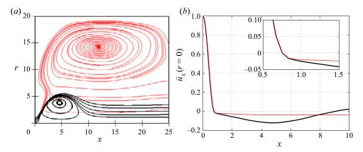
Figure 10. Comparison of time-averaged flow features for S = 2.1 using (a) projected streamlines on meridional plane and (b) centreline axial velocity variation (inset showing variation in the vicinity of the stagnation point), for conical form of vortex breakdown (CVB) types: \_\_\_\_\_\_, black (thick), regular; \_\_\_\_\_\_, red (thin), wide-open.
