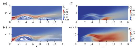
Figure 5. Time-averaged features based on azimuthally-averaged fields with (*a*) projected streamlines on meridional plane and axial mean velocity contours and (*b*) contours of rms of the fluctuating axial velocity field shown for cases S = 1.3 (*a*,*b*) and S = 1.4 (*c*,*d*).
