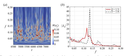
Figure 15. (a) Scalogram showing the magnitude of the continuous wavelet transform of  $u'_y$  for x = y = 6 and z = 0 for conical form of vortex breakdown (CVB) at S = 1.5. (b) Variation of the dominant eigenvalue from spectral proper orthogonal decomposition,  $|\lambda_1(f)|$ , with the frequency is shown for bubble form of vortex breakdown (BVB) at different swirls.
