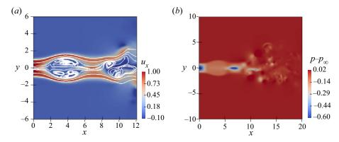
Figure 2. Instantaneous flow features of bubble form of vortex breakdown (BVB) at S = 1.3 shown on the z = 0 plane using (*a*) projected streamlines overlaid on axial velocity contours and (*b*) pressure contours.
