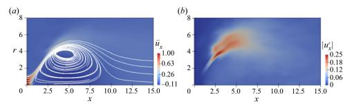
Figure 7. Time-averaged flow structure of regular conical form of vortex breakdown (CVB) at S = 1.8 on meridional plane: (*a*) projected streamlines overlaid on contours of mean axial velocity and (*b*) rms of the fluctuating axial velocity component.
