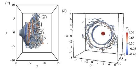
Figure 6. Three-dimensional spatial structure of regular conical form of vortex breakdown (CVB) for S = 1.8, visualized using isosurfaces of (*a*) vorticity magnitude,  $|\omega| = 1.5$  and (*b*)  $\lambda_2 = -2$ . Inflow swirl is clockwise (see § 2) implying a counter-winding spiral vortical structure.
