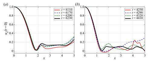
Figure 4. Axial velocity variation along the swirling jet axis for the bubble form of vortex breakdown (BVB) at different time instants and for (a) S = 1.3 and (b) S = 1.4.
