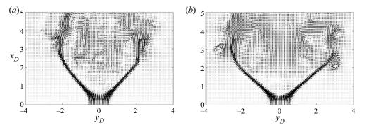
Figure 17. Projected velocity vectors on z = 0 plane at arbitrary instants for (*a*) S = 1.4 and (*b*) S = 1.45, showing regular conical form of vortex breakdown (CVB). These flow states closely resemble that reported in Liang & Maxworthy (2005) (length scale changed to jet diameter, i.e.  $x_D = x/2$ , for ease in comparison).
