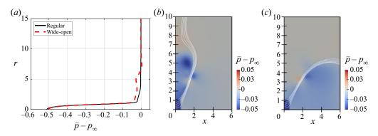
Figure 18. Time-averaged pressure for bistable types of conical form of vortex breakdown (CVB) at S = 2.1: (*a*) comparison of profiles at inflow (x = 0) as a function of radial distance of bistable states at S = 2.1; contours on the meridional plane for (*b*) wide-open type and (*c*) regular type (projected streamlines based on mean flow shown for reference and contour range reduced in extent for clarity).
