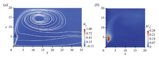
Figure 9. Time-averaged flow features for wide-open conical form of vortex breakdown (CVB) at S = 2.15: (*a*) projected streamlines and contours of  $u_x$  and (*b*) rms of fluctuating axial velocity on meridional plane.
