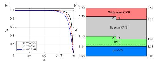
Figure 1. (a) Variation of the transfer function with wavenumber for tenth-order filter and different  $\alpha_f$ . (b) Schematic showing the extended ranges of existence of various VB flow states observed for Re = 1000. The dashed line at S = 1.2 shows the upper limit of the range where |m| = 4 structures are observed. Arrows indicate the sense in which S is changed in the hysteresis studies.
