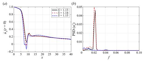
Figure 21. (a) Time-averaged centreline axial velocity and (b) periodogram of the fluctuating axial velocity component at x = 7 on the axis.
