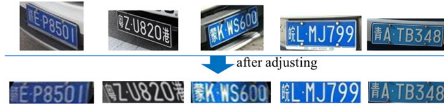
Fig. 2. The correct results after license plate adjusting.
