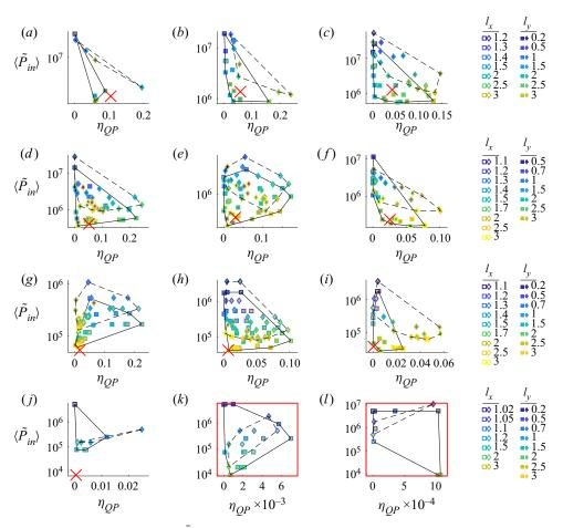
Figure 17. Values of  $\eta_{QP}$  versus  $\langle \tilde{P}_{in} \rangle$  for rectangular (coloured squares) and rhombic lattices (coloured diamonds), at various  $l_x$  and  $l_y$  (colours at right). The values for isolated flapping plates are shown by red crosses (where self-propelled states occur). From the top to bottom rows, Re = 70, 40, 20 and 10. From the left to right columns, A/L = 0.2, 0.5 and 0.8.
