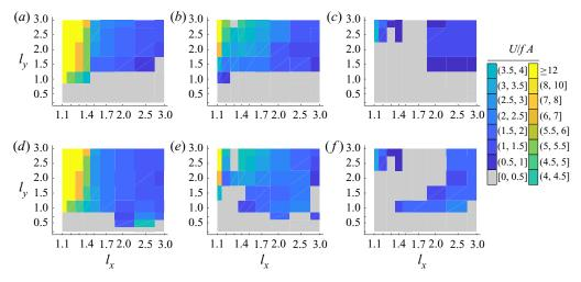
Figure 13. Comparison of self-propelled speeds for rectangular (a-c) and rhombic (d-f) lattices at Re = 20 and A/L = 0.2 (a,d), 0.5 (b,e) and 0.8 (c,f).
