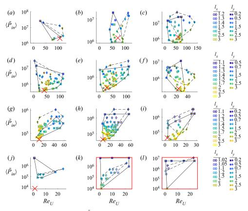
Figure 16. Values of  $Re_{U,SPS}$  versus  $\langle \tilde{P}_{in} \rangle$  for rectangular (coloured squares) and rhombic lattices (coloured diamonds), at various  $l_x$  and  $l_y$  (colours at right). The values for isolated flapping plates are shown by red crosses (where self-propelled states occur). From the top to bottom rows, Re = 70, 40, 20 and 10. From the left to right columns, A/L = 0.2, 0.5 and 0.8.
