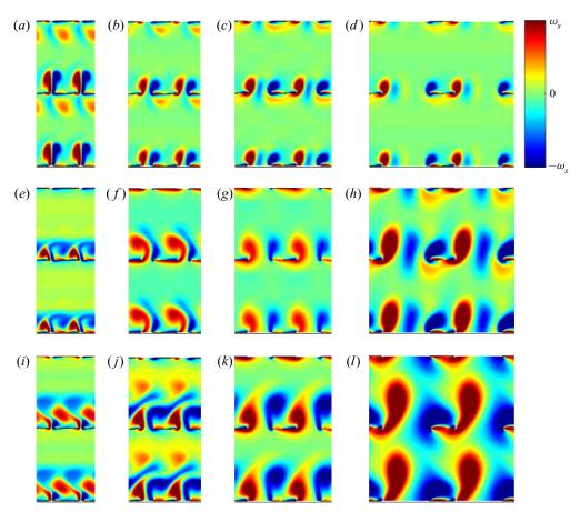
Figure 10. Flow snapshots with  $l_x = 1.2$ , 1.5, 2 and 3 (left to right columns) and A/L = 0.2, 0.5 and 0.8 (top to bottom rows). The other parameters are: Re = 20, U/fA = 3,  $l_y = 3$ . The colour bar limits are  $\pm \omega_s$  where  $\omega_s = 30$  (a), 20 (b), 10 (c,d), 100 (e), 50 (f), 30 (g), 10 (h), 150 (i), 50 (j), 30 (k) and 10 (l).
