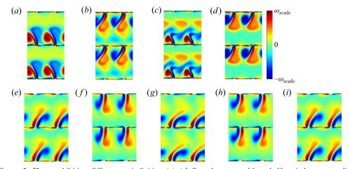
Figure 5. Flows exhibiting different periodicities. (*a*)–(*d*) Snapshots spaced by a half-period corresponding to  $F_x(t)$  in figure 4(*d*). Panel (*d*) is essentially a mirror image of panel (*a*). (*e*)–(*i*) Snapshots spaced by a half-period for a 2-periodic flow (Re = 20, A/L = 0.5,  $l_x = 1.3$ ,  $l_y = 2$  and U/fA = 3). The colour bar limits are  $\pm \omega_{scale}$  where  $\omega_{scale} = 300$  (*a*–*d*) or 100 (*e*–*i*).
