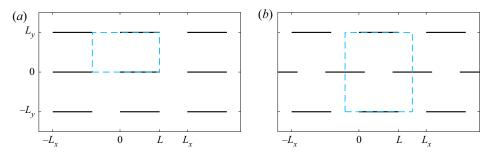
Figure 1. (a) A rectangular lattice of plates. The computational domain is an  $L_x$ -by- $L_y$  unit cell, shown with a dashed blue outline. (b) A rhombic lattice of plates. The computational domain is an  $L_x$ -by- $2L_y$  double unit cell, shown with a dashed blue outline.
