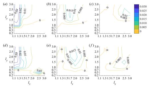
Figure 12. Contours of Froude efficiency for rectangular (a-c) and rhombic lattices (d-f) at A/L = 0.2 (a,d), 0.5 (b,e) and 0.8 (c,f).
