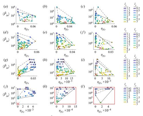
Figure 15. Peak values of  $\eta_{Fr}$  versus  $\langle \tilde{P}_{in} \rangle$  for rectangular (coloured squares) and rhombic lattices (coloured diamonds), at various  $l_x$  and  $l_y$  (colours at right). The values for isolated flapping plates are shown by red crosses (where  $\eta_{Fr} > 0$ ). From the top to bottom rows, Re = 70, 40, 20 and 10. From the left to right columns, A/L = 0.2, 0.5 and 0.8.
