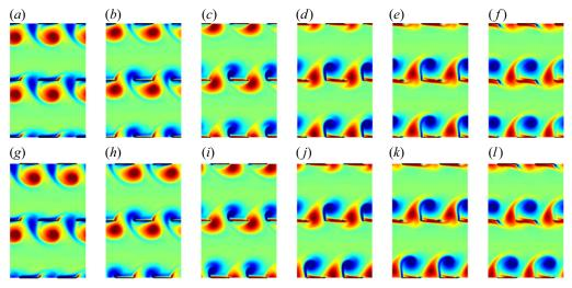
Figure 9. Six vorticity snapshots spaced by 0.1 in *t* during the half-period of upward flow, for rectangular (a-f) and rhombic (g-l) lattices. The parameters are A/L = 0.5,  $l_x = 2$ ,  $l_y = 3$ , Re = 70 and U/fA = 7.
