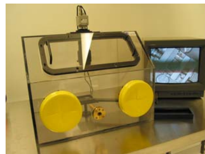
Fig. 2. The custom inert gas Glove Box with video camera and video monitor
