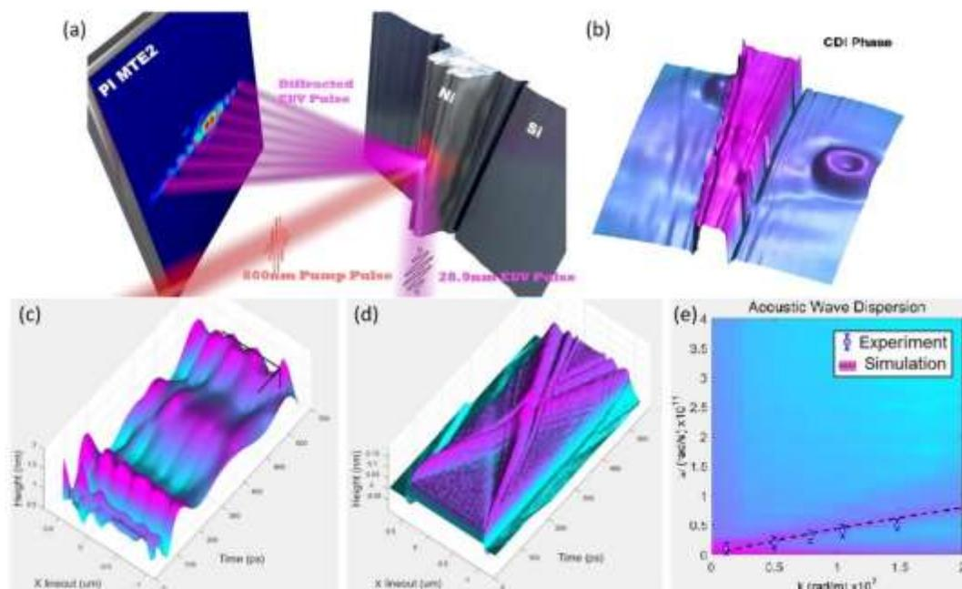
**Figure 1.** (a) Experimental setup for full field EUV dynamic imaging on a tabletop. (b) Phase image of a nanostructured nickel triangle taken using coherent diffractive imaging. (c) Lineout of the height of the nanostructure as a function of pump probe delay. (d) Simulation of the time evolution of a 2.2 $\mu$ m cross-section of the nickel triangle after impulsive heating. (e) The dispersion relation of the acoustic waves launched by the pump pulse.
