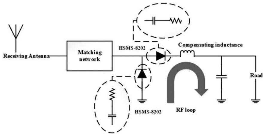
Fig. 7. The series-parallel rectifier with an inductance loaded.
