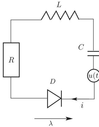
FIGURE 1. A circuit with an ideal diode and a voltage source.
