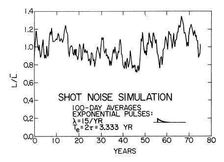
Fig. 5. Typical shot noise generated by computer, consisting of random exponentially-decaying pulses, as shown, with rate and pulse length  $T_e$  similar to 3C 273 parameters.
