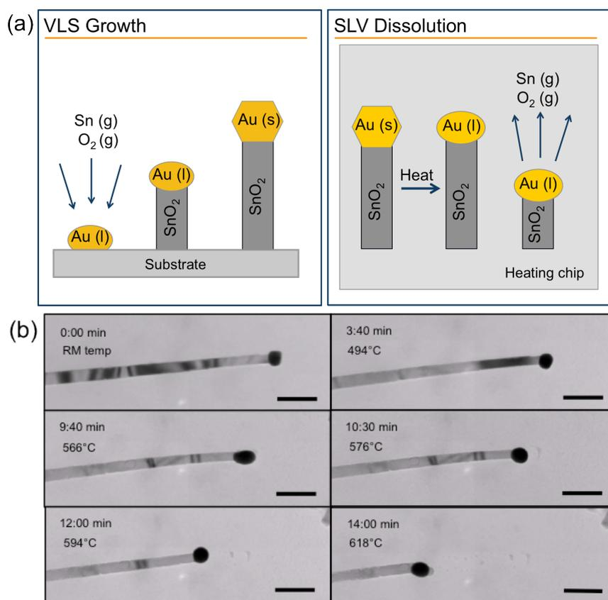
**Figure 1.** (a) Cartoon showing the relation between VLS nanowire growth and SLV dissolution of a SnO<sub>2</sub> nanowire. (b) Snapshots from a movie recorded during heating of a SnO<sub>2</sub> nanowire showing dissolution occurring at elevated temperature. Scale bar equals 0.2  $\mu\text{m}$ .
