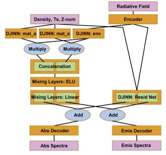
FIGURE 2. This is the full architecture as described. Excluded from this diagram are the locations and types of transformation operations.
