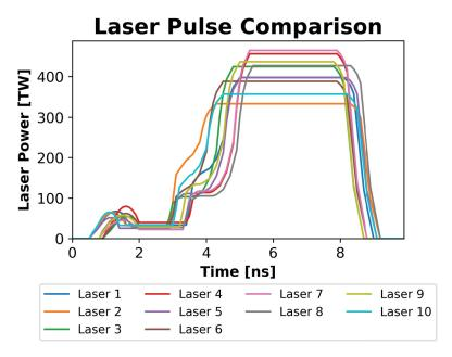
FIGURE 3. These are the ten laser profiles used in the simulations. They are randomly generated perturbations to the profile of the N210808 shot at the National Ignition Facility (Callahan 2021).
