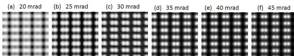
**Figure 2.** Simulated dark-field images of the Ge [112] specimen at convergence semi-angles of (a) 20 mrad, (b) 25 mrad, (c) 30 mrad, (d) 35 mrad, (e) 40 mrad, and (f) 45 mrad at 60 kV [7] by the multi-slice method.
