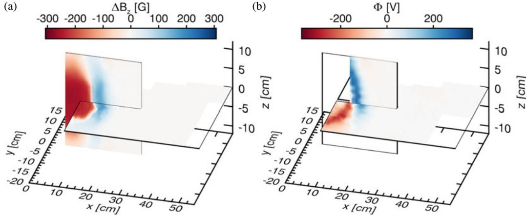
**Figure 3.** Composite plots of (a) the magnitude of the relative magnetic field  $\Delta B_z = B_z - B_0$  and (b) the electrostatic potential  $\Phi$  in the  $x$ - $z$  and  $x$ - $y$  planes at the same time  $t = 0.5 \mu\text{s}$ . Each plane is comprised of thousands of separate laser shots, showing a high degree of reproducibility. The target is located at  $\{x, y, z\} = \{0, 0, 0\}$ .
