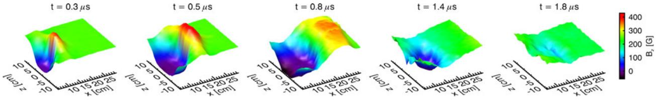
**Figure 4.** Time series of surface plots of  $B_z$  in the  $x$ - $z$  plane, where the vertical dimension (color) is the magnitude of  $B_z$ . The target is at  $\{x, z\} = \{0, 0\}$  and the background field  $B_0 = 250 \text{ G}$  along  $\hat{z}$ .
