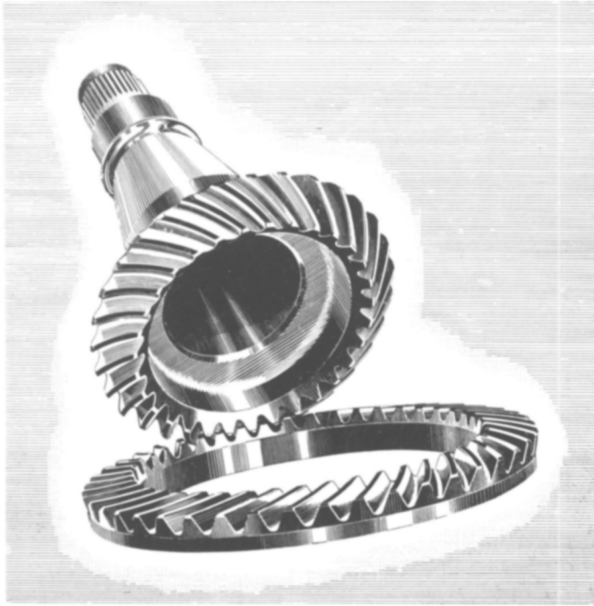
ENV spiral bevel gears used in Westland S 55 main rotor drive
