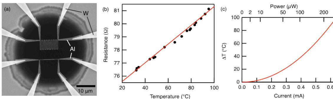
**Figure 2.** (a) Scanning electron microscope image of a serpentine heater (top) and thermometer (bottom) patterned with 50-nm thick Al. (b) Thermometer resistance as a function of temperature, where the line is a linear fit to the experimental data points. (c) Temperature rise at the heater calculated as a function of serpentine heater current assuming cylindrical geometry and a liquid/membrane total thickness of 200 nm with composite thermal conductivity of 1.5 W/(m K).
