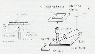
The flat pH imaging sensor enables the pH distribution in a semi-solid electrolyte solution, such as agar film, to be detected and observed. Placing solid samples in contact with the agar film contact with the agar film contact with the agar film contact be solutions that indirectly describes the surface condition or even the inner condition of the contact solid sample.
