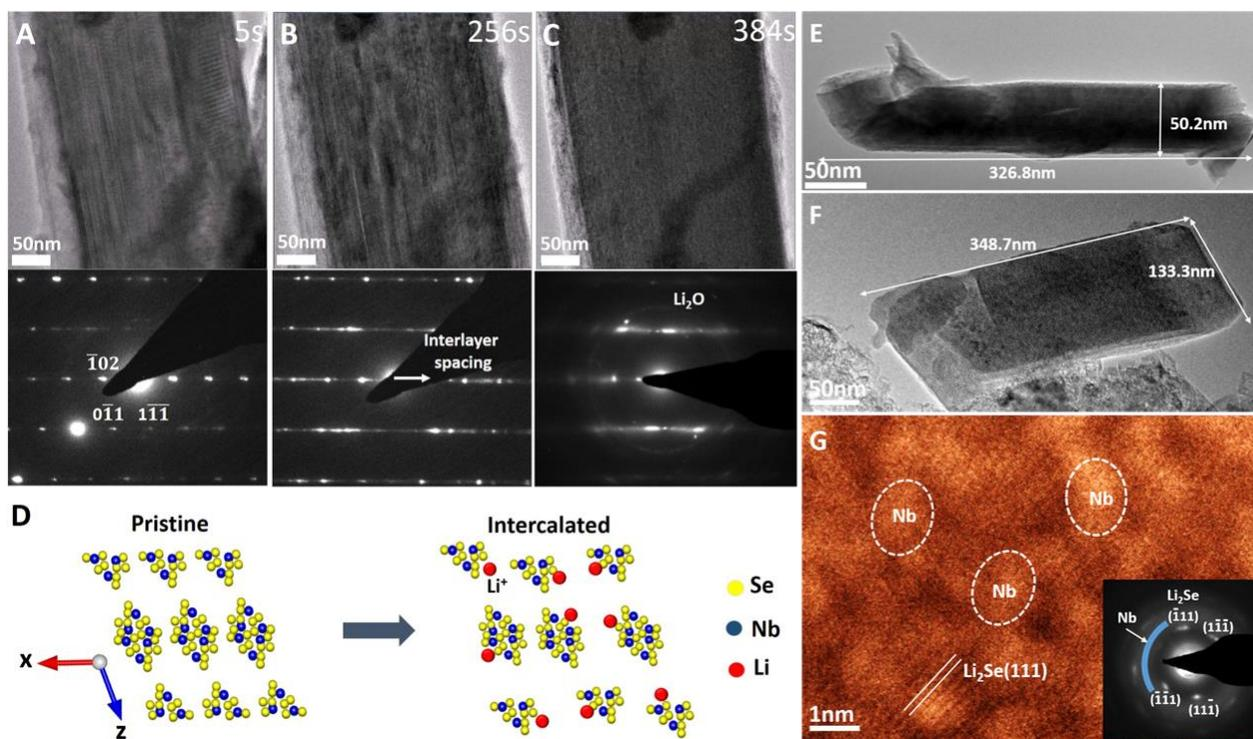
**Figure 1.** A)-B) Time-resolved TEM images show the lithiation process of a large NbSe<sub>3</sub> ribbon. D) Schematic of intercalation of NbSe<sub>3</sub>. A small pristine D) and lithiated E) NbSe<sub>3</sub> ribbon. G) HAADF STEM images of the lithiated small NbSe<sub>3</sub> ribbon showing the Nb metal particles embedded in the Li<sub>2</sub>Se matrix.
