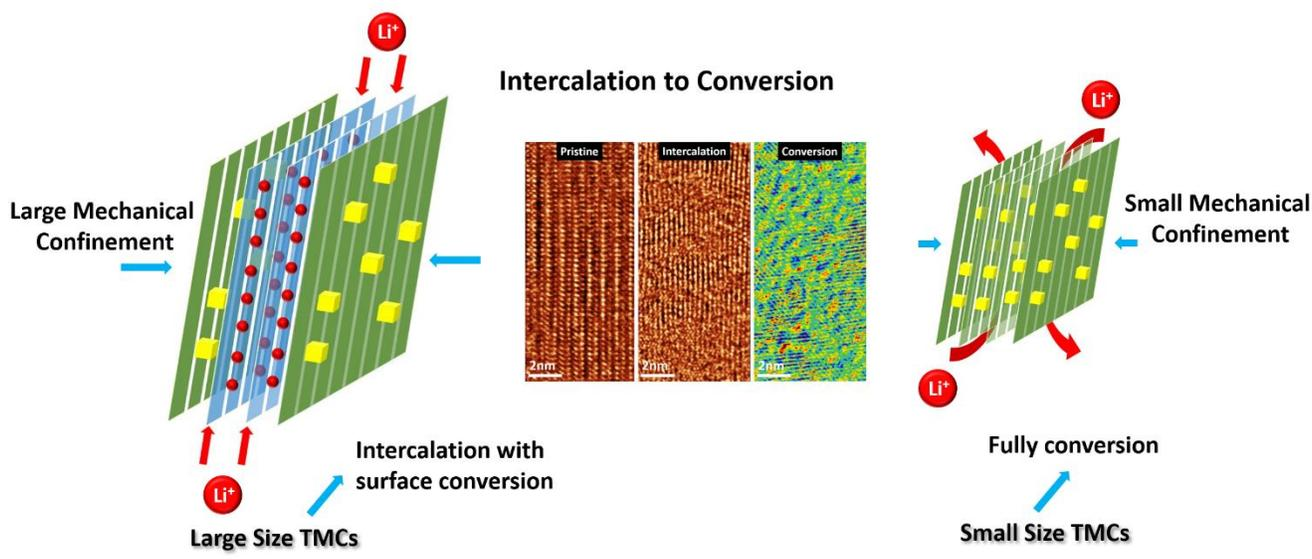
**Figure 2.** Schematic drawings to illustrate the size effect on the lithiation reaction mechanisms: the large size TMC is dominated by intercalation reaction and the surface region is subjected to conversion reaction; while the small size TMC is fully converted upon lithiation.
