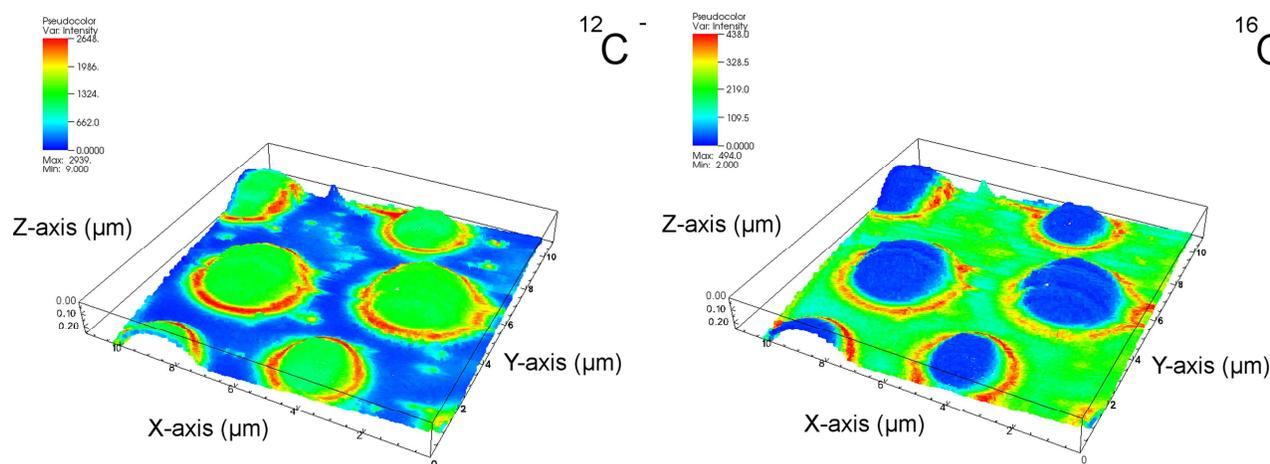
**Figure 2.** PS/PMMA blend (Field of view:  $22.3 \times 17.3 \mu\text{m}^2$ ): (a) Combined SIMS-SPM 3D reconstruction of the  $^{12}\text{C}^-$  secondary ion signal. (b) Combined SIMS-SPM 3D reconstruction of the  $^{16}\text{O}^-$  signal, which is characteristic of PMMA [3].
