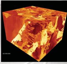
Austenic-ferritic duplex steel, 16 x 12 x 18 µm³ volume acquired with the AutoSlice and View™ application. A series of top-down high energy, high angle SEM-BSE images were collected automatically. The distance between each slice is 30 nm. Courtesy of FEI NanoPort.
