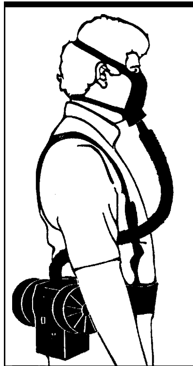
FIGURE. Example of a NIOSH-certified, powered HEPA-filter halfmask respirator (MSA OptimAir 6A, NIOSH approval TC-21C-513).
