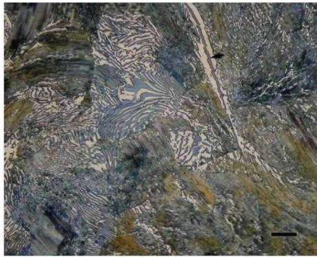
Figures 14 and 15: Cartridge brass micrograph shown in Figures 6 and 7 tint etched with Beraha's PbS reagent (left) and cementite in a hot rolled Fe-1% C binary alloy colored with Beraha's sodium molybdate reagent (right). Magnification bars are 200 and 20 \mu\text{m} , respectively.
