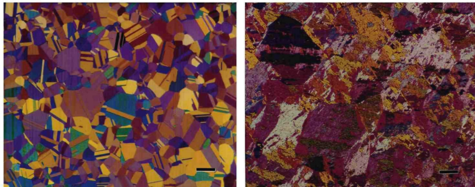
Figures 10 and 11: FCC twinned grain structure of heading quality Custom Flo 302 stainless steel revealed using Beraha's B1 reagent and lath martensite grain structure of over-austenitized (1093 ^{\circ}\text{C} ) AerMet 100 ultra-high strength steel revealed using 10% sodium metabisulfite. Both viewed with polarized light plus sensitive tint. The magnification bars are 100 \mu m long.
