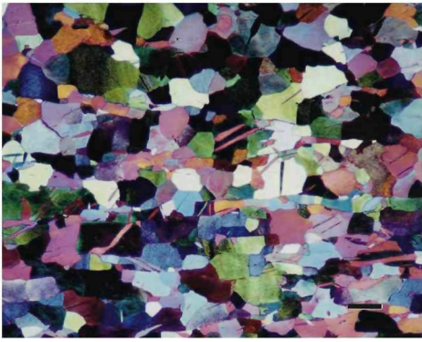
Figures 20 and 21: Grain structure of as-rolled CP Ti (ASTM F67, Grade 2) containing mechanical twins (left) etched with modified Weck's reagent and cold rolled pure molybdenum (right) colored with the reagent developed by Oak Ridge National Laboratory. Magnification bars are 100 and 20 \mu\text{m} long, respectively.
