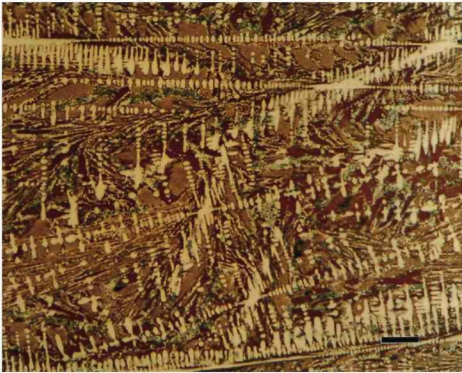
Figures 16 and 17: Cementite in the chill cast surface of gray iron etched with Beraha's selenic acid reagent for cast iron (left) and twinned FCC alpha phase and beta phase (mottled and outlined) in Cu-40% Zn revealed using Beraha's selenic acid reagent for copper alloys. Magnification bars are 50 and 20 \mu\text{m} long, respectively.
