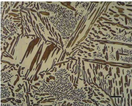
Figures 18 and 19: Austenite colored in ASTM A890 Grade 5A cast duplex stainless steel with the LB1 reagent (left) and the cast grain structure of 206 aluminum revealed using Weck's reagent for Al alloys (right). The magnification bars are 100 and 50 \mu\text{m} long, respectively.
