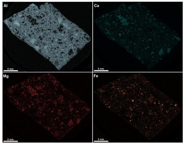
**Figure 1.** Montage EDS maps of an entire 2.5 x 1.5 cm Hornblende Basalt section acquired using EDAX APEX 2.0 software show heterogeneity.
