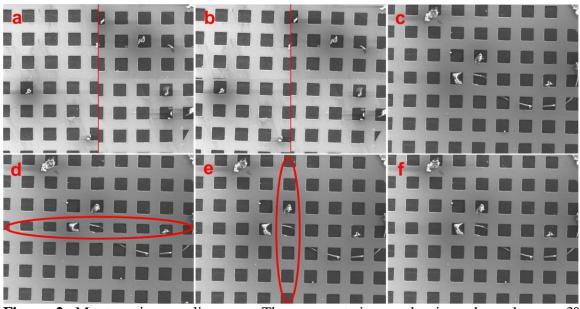
**Figure 2.** Montage image alignment. The scan rotation angles in a, b, and c are 3°, 1°, and 1.6°, respectively. 1.6° represents a good scan rotation calibration without mismatch in the figure.
