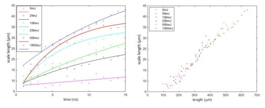
Figure 11. The density scale lengths versus time (left) and blast wave radii length (right), for density of  $n = 4.52 \times 10^{21}$  cm<sup>-3</sup> and absorbed energies of 5, 50, 100, 250, 500 and 1000 mJ.
