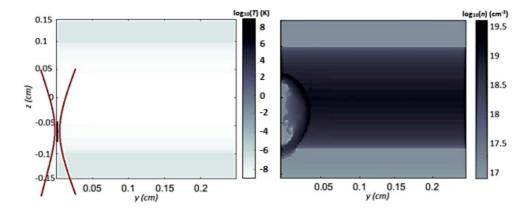
Figure 3. Left: the cylinder where the energy is deposited, representing the confocal volume of the laser pulse with  $w_0 = 35 \,\mu\text{m}$  and  $Z_R = 374 \,\mu\text{m}$ . At t = 0, the beam is focused at z = -0.06 cm along the laser propagation axis (z-axis) along the direction of the gas flow (y-axis). Right: the formation of the blast wave at t = 4 ns corresponding to the CO<sub>2</sub> specifications, at 4 bar initial pressure and absorbed energy 100 mJ, deposited at z = -0.02 cm.
