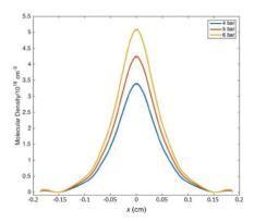
**Figure 5.** The profiles of backing pressures of 4, 5 and 6 bar (maximum) that correspond to the molecular densities of  $n = 3.39 \times 10^{18} \text{ cm}^{-3}$ ,  $n = 4.42 \times 10^{18} \text{ cm}^{-3}$  and  $n = 5.09 \times 10^{18} \text{ cm}^{-3}$ , respectively.
