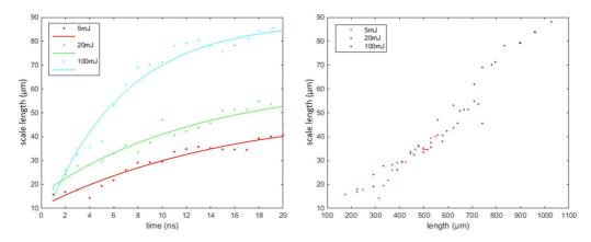
Figure 9. The density scale lengths versus time (left) and blast wave radii length (right), for density of  $n = 4.42 \times 10^{18}$  cm<sup>-3</sup> and absorbed energies of 5, 20 and 100 mJ.
