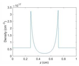
Figure 1. Simulation of the spherical expansion of the blast wave (left) and the lineout (red line) of the steep density walls at the front of the shock (right) in an homogeneous hydrogen gas, for initial density of  $0.5 \times 10^{17}$  cm<sup>-3</sup> and 1 mJ absorbed energy of the BNL CO<sub>2</sub> laser.
