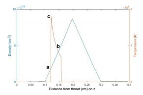
**Figure 4.** The triangular density shape used in the simulation (blue) and the initial energy deposition (red), for  $w_0=35~\mu m,~Z_R=374~\mu m$  and  $E_{\rm abs}=10~{\rm mJ}.$
