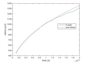
**Figure 6.** Comparison of the FLASH and self-similar Sedov results for 20 mJ absorbed energy, for initial density  $n = 3.39 \times 10^{18}$  cm<sup>-3</sup>, deposited at 0.02 cm prior to the centre of the throat.
