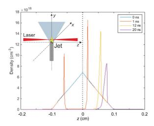
**Figure 2.** Time evolution of density profiles along the laser propagation axis for a blast wave at t=0,1,12 and 20 ns, corresponding to the BNL CO<sub>2</sub> laser, at 4 bar initial pressure and absorbed energy 20 mJ. The laser beam is focused at z=-0.02 cm.
