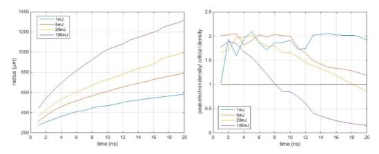
Figure 8. The blast wave radii (left) and the corresponding ratio of the peak electron density to the critical density (right). Time evolution up to 20 ns for 1, 5, 20 and 100 mJ absorbed energy deposited at 0.02 cm prior to the centre of the throat. Initial density was set to  $n = 3.39 \times 10^{18}$  cm<sup>-3</sup>.
