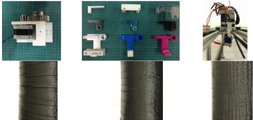
**Figure 6.** An example of iterative design. (Left) Initial design; (centre) a series of three iterative refinements; (right) the final design for a large-scale 3D printer extrusion head. The reliability of the print process gradually increased with each iteration (test prints shown below each design). The final design required nearly 40 iterations to achieve reliable printing. Courtesy of Gilmour Space Technologies.
