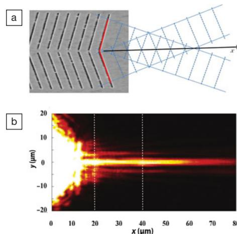
A cosine-Gauss plasmon beam, dubbed a “needle beam,” propagates without diffraction; (a) a micrograph and diagram of the metallic gratings that produce the needle beam and (b) experimental results. *Courtesy of Patrice Genevet.*
