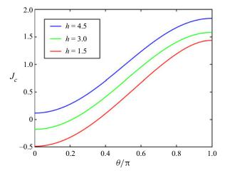
Figure 5. Condensation flux as a function of the scaled vertical coordinate for L = 0.0514,  $\gamma = 14.3$ , k = 0.0413,  $\hat{G}_c = 287 \text{ m}^{-1}$ , and different droplet locations. The bottom of the droplet corresponds to  $\theta = \pi$ .
