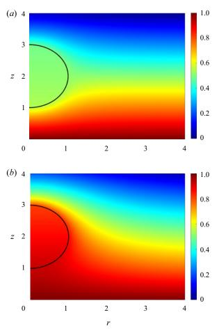
Figure 4. Solutions for the temperature in both moist air and liquid for (*a*) the model that neglects phase change at the droplet surface, and (*b*) the model with L = 0.0514,  $\gamma = 14.3$ , based on levitation experiments with microscale water droplets (Zaitsev *et al.* 2021). For both cases, k = 0.0413 and  $\hat{G}_c = 287 \text{ m}^{-1}$ .
