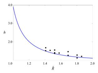
Figure 3. Comparison of the predicted levitation height with experimental data at 63 °C from Zaitsev *et al.* (2021). The blue curve is predicted by the theory, with  $\hat{G}_c = 287 \text{ m}^{-1}$  and the same values of other non-dimensional parameters as in the previous figure. Filled squares represent experimental measurements based on optical recordings of size and location of levitating droplets, expressed in our non-dimensional variables.
