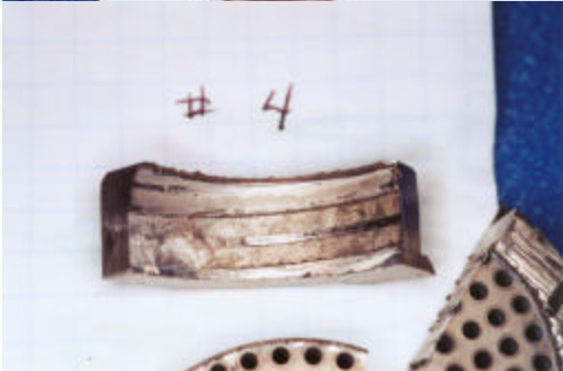
Figures 3 and 4. Optical photographs showing how the sections were removed for SEM examination and cross section. Also showing the brazing joint fracture.
