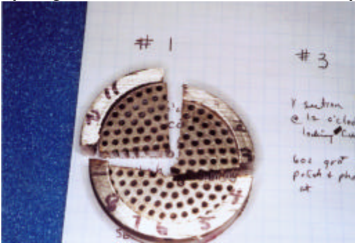
Figure 2. An optical photograph of the hydrogen inlet tubesheet braze assembly.
