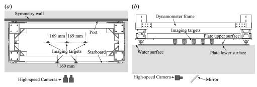
Figure 4. Top and side views of the set-up for the free vibration experiments are shown in (a,b), respectively. In the depicted configuration, the lower side of the plate is slightly below the water surface while the upper side is dry. The carriage structure above the dynamometer frame is omitted.
