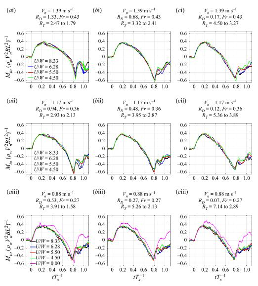
Figure 9. The dimensionless transverse moment about the plate's centre,  $M_{to}^* = M_{to}(\rho_w V_n^2 B L^2)^{-1}$ , vs  $t/T_s$  is plotted for the same conditions as in the corresponding plots of  $F_n^*(t/T_s)$  in figure 8. See the caption to figure 8 for additional details. Results are shown for (*a*i)–(*a*iii) h = 6.61 mm, (*b*i)–(*b*iii) h = 8.27 mm, (*c*i)–(*c*iii) h = 13.22 mm.
