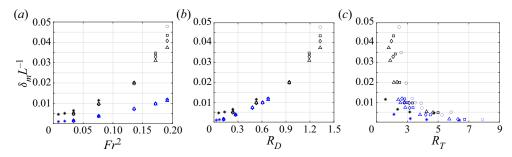
Figure 26. The maximum dimensionless out-of-plane deflection at the plate centre,  $\delta_m L^{-1}$ , for all impact conditions vs  $Fr^2$  (subplot *a*),  $R_D$  (subplot *b*) and  $R_T$  (subplot *c*). Symbol definitions: black -h = 6.61 mm; blue -h = 8.27 mm.  $\circ - U/W = 8.33$ ;  $\Box - U/W = 6.28$ ;  $\diamond - U/W = 5.50$ ;  $\Delta - U/W = 4.50$ ; \* - U/W = 0.00.
