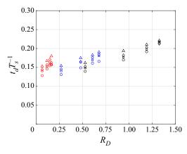
Figure 22. The dimensionless delay time at spray root emergence from the leading edge of the plate,  $t_d/T_s$ , vs  $R_D$ . The definition of  $t_d$  is given in the caption of figure 21. Plotting symbol definitions: black -h = 6.61 mm; blue -h = 8.27 mm; red -h = 13.22 mm;  $\circ -U/W = 8.33$ ;  $\Box -U/W = 6.28$ ;  $\diamond -U/W = 5.50$ ;  $\Delta -U/W = 4.50$ .
