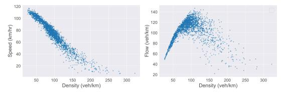
*Figure 2.* Figures showing the empirical relationship between vehicle flow q, density ρ, and velocity v. The data is taken from detectors on the M25 measuring various quantities averaged every minute.
