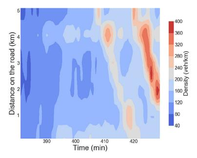
**Figure 1.** Density estimated from occupancy for the section of M25 on January 8, 2007 between 6:21 am and 7:09 am. We observe forward moving free flow waves between minutes 381 and 405, which correspond to the movement of vehicles. We also observe backward moving high-density waves in the second half of the x - t plane.
