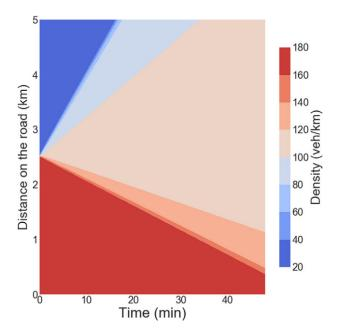
**Figure 4.** The Riemann Problem with  $\rho_{i-1} > \rho_i$  causes a rarefaction wave. The initial condition (namely at t = 0) consists of a constant value of high density for  $x \in [0, 2.5]$  and a constant value of low density for  $x \in [2.5, 5]$ . As the simulation moves forward in time we observe a rarefaction wave, or a fanning out of density values between the low and high values of the initial condition.
