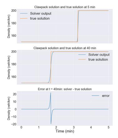
**Figure 5.** We plot the analytic solution to the Riemann Problem along with its numerical solution using Clawpack. As time progresses we observe that the discontinuity is smoothed slightly. However, we notice that the position of the shock wave remains accurate.
