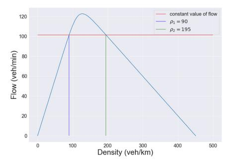
*Figure 15.* Del Castillo fundamental diagram. The two vertical lines correspond to two values of density ( $\rho_1 = 90$  and  $\rho_2 = 195$ ) that map to the same value of flow. As the likelihood is built from flow, these two values of density are equally likely and therefore the posterior exhibits multimodality.
