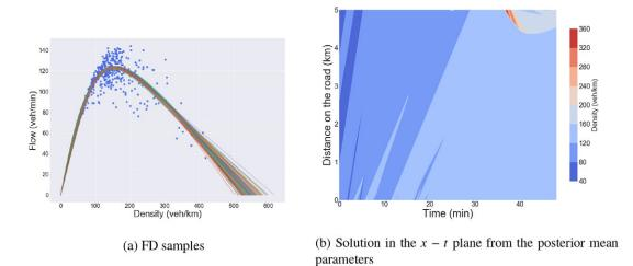
**Figure 8.** Posterior samples from a direct fit of del Castillo's fundamental diagram (FD) to M25 data. (a) Plotted FDs using the samples. (b) Density in the x - t plane from Lighthill–Whitham–Richards. Parameters used are the posterior mean from samples. We notice that the congested flow waves do not cross the domain as they do in the data.
