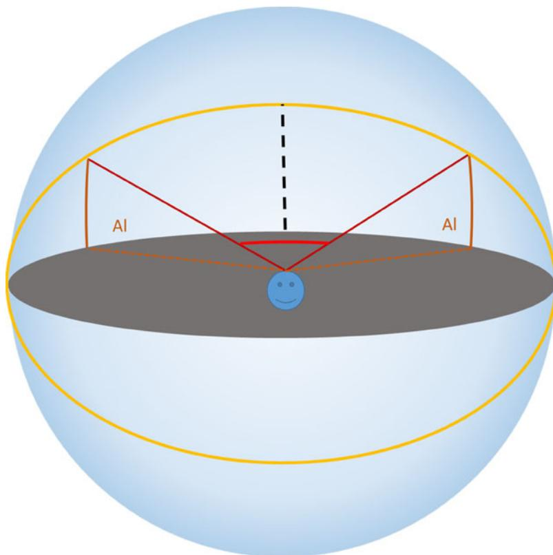
**Figure 3.** The observer takes sights on the celestial body as it passes through the fixed-angle of the Bris sextant ascending, then descending. By knowing the altitude and timing of the observations and the declination of the celestial body, it is possible to derive latitude (the height of the black line) and longitude (the East–West position of the black line) using the methods proposed here.
