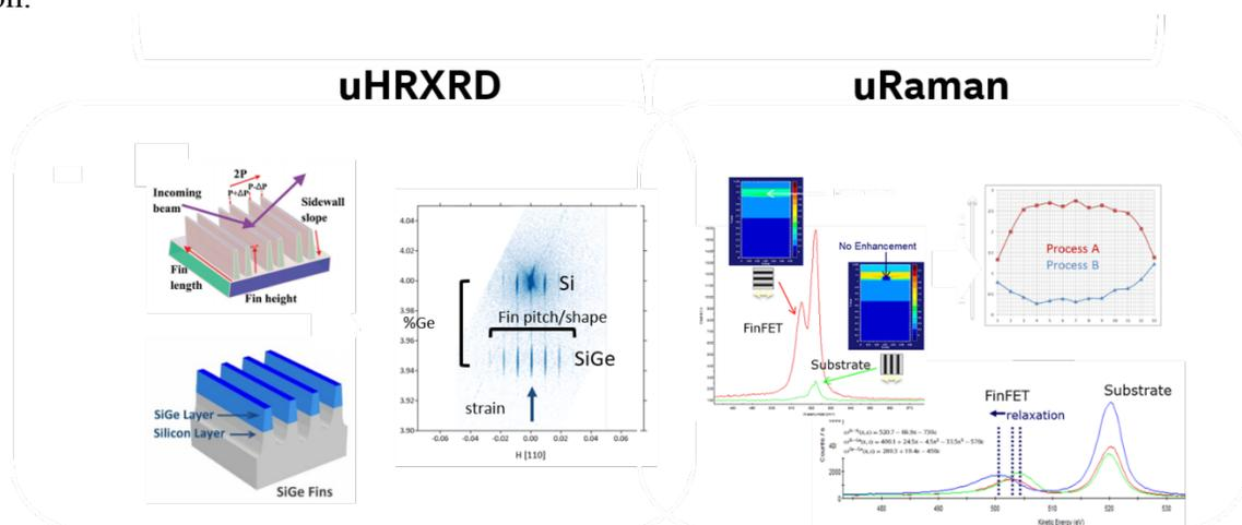
**Figure 2.** X-ray diffraction of tri-gate array structure (left). Raman spectroscopy (right) of tri-gate showing field enhancement effect from data and simulation and the capability of mapping the localized strain across a wafer.
