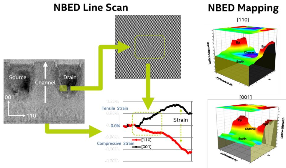
**Figure 1.** (Left) NBED strain line scan profile shows the strain sensitivity to nearby source/drain microstructure. (Right) NBED strain map of a tri-gate transistor in [110] channel direction and [001] direction.
