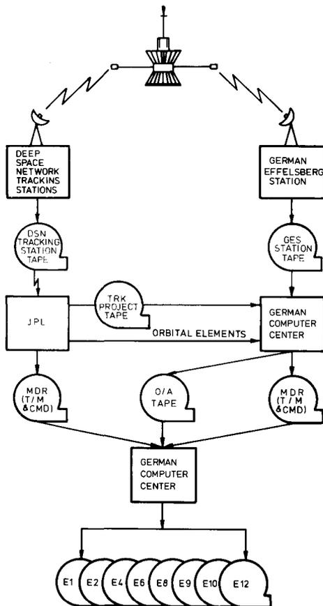
Figure 3 - Helios System Data Flow
