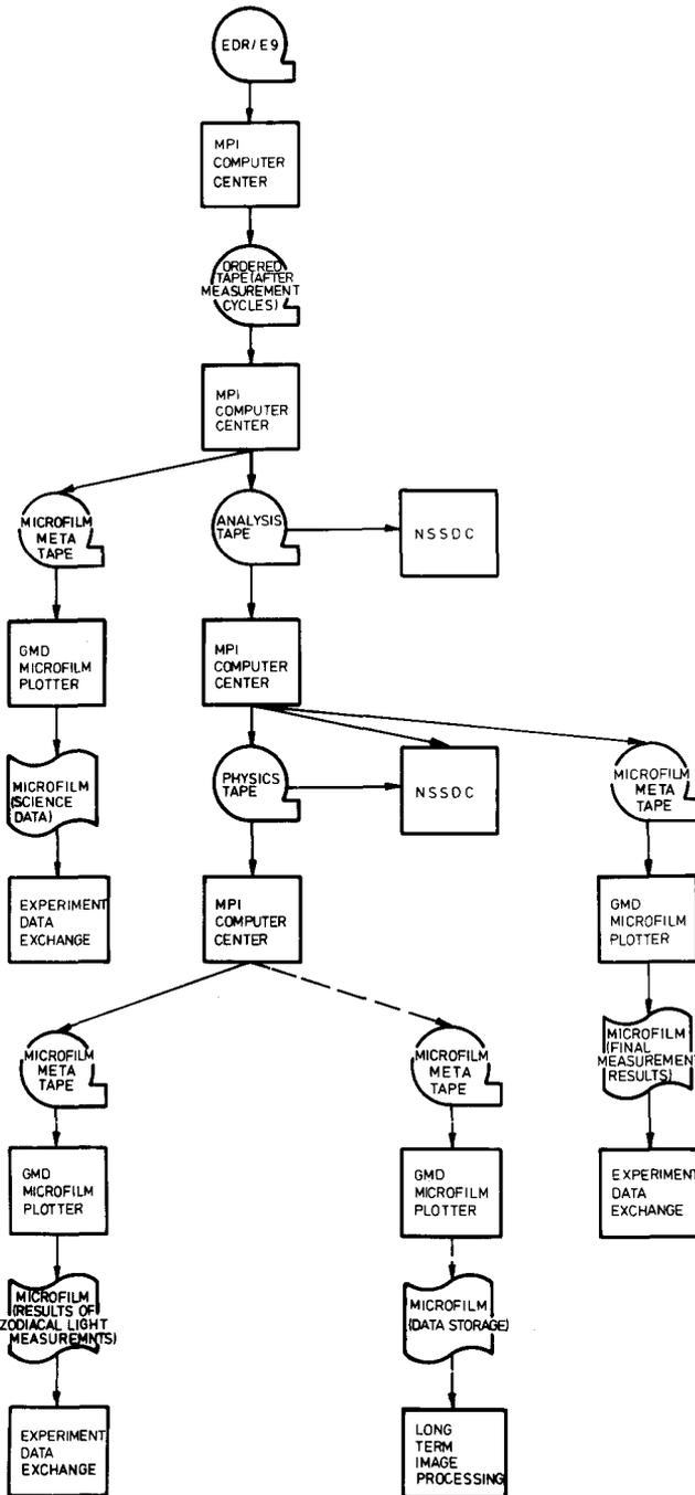
Figure 4 - Zodiacal Light Experiment System Data Flow
