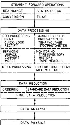
Figure 2 - Experimenter Data System-Processing Levels
