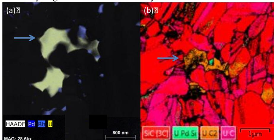
**Figure 1.** (a) STEM/EDS map of fission product precipitates at the boundaries of SiC grains. In this example, from the as-irradiated particle, uranium is shown both co-located with metallic fission products Pd and Rh, and on its own. (b) Is a tKD Euler micrograph of the same region, as indicated by the blue arrows. Preliminary results indicate UC<sub>2</sub> as the bulk uranium precipitate.
