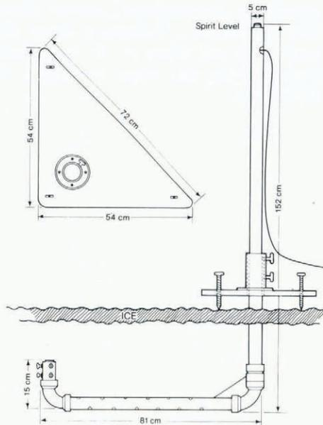
Fig. 1. Design details of the support arm for the underwater sensor.
