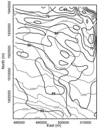
Fig. 4. Snow accumulation map  $(kg m^{-2} a^{-1})$  by snow radar (third layer, 366 year average) and surface topography (grey line). Map projection in UTM (WGS84).
