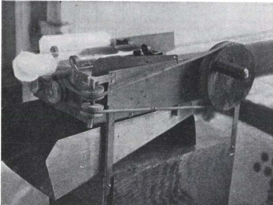
Fig. 1. Hand-driven rolling machine.
