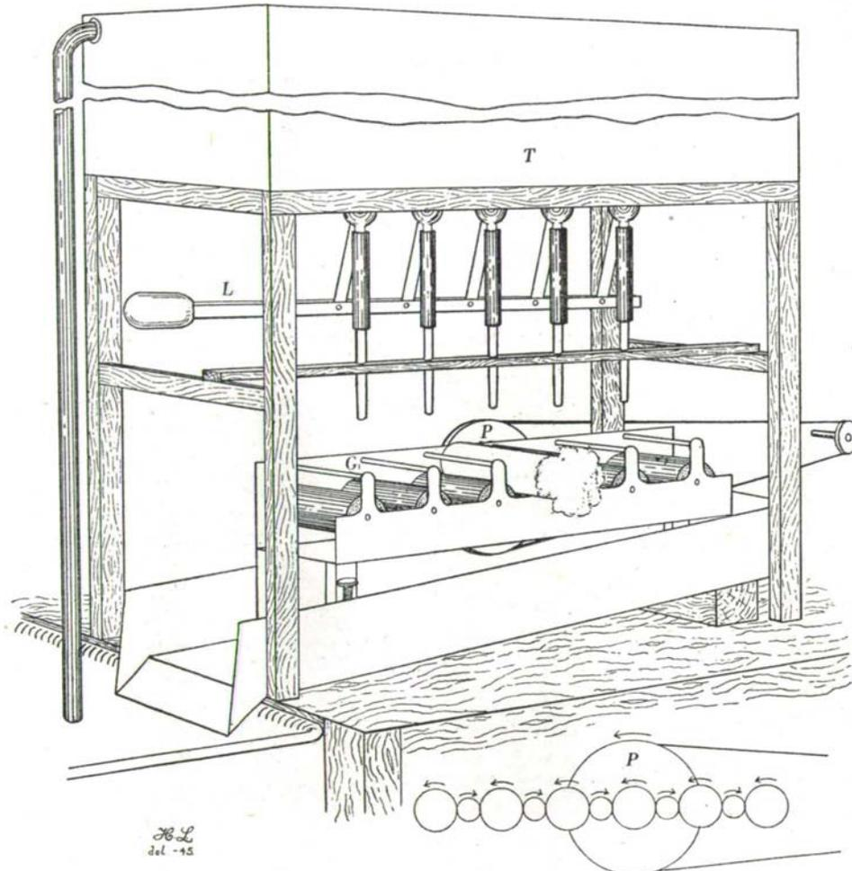
Fig. 2. Rolling machine for five tubes, showing one in position. Inset below: diagram of gears. *T*, water tank; *L*, lever controlling taps; *P*, driving pulley; *G*, guard rail to prevent displacement of tubes.
