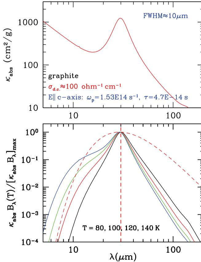
**Figure 3.** Upper panel: the opacity of graphite with a d.c. conductivity of  $\sigma_{d.c.} = 100 \text{ ohm}^{-1} \text{ cm}^{-1}$ . A prominent  $30 \mu\text{m}$  feature with a FWHM of  $\sim 10 \mu\text{m}$  is clearly seen. Lower panel: the emission profiles of graphite with  $\sigma_{d.c.} = 100 \text{ ohm}^{-1} \text{ cm}^{-1}$  at  $T = 80, 100, 120, 140 \text{ K}$ . Dot-dashed line: the  $T = 100 \text{ K}$  blackbody.
