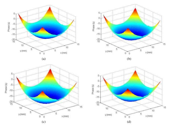
Figure 3. Wavefront distributions associated with the vapor cell when the temperatures of the heater are (a)  $60^{\circ}$ C, (b)  $80^{\circ}$ C, (c)  $100^{\circ}$ C and (d)  $120^{\circ}$ C, respectively.
