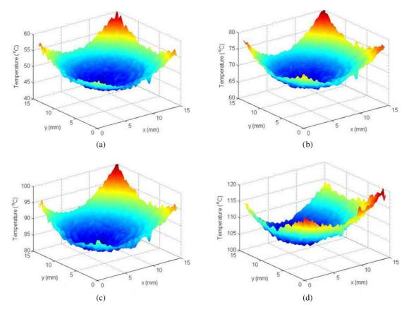
Figure 5. Temperature distributions at the cross-section of a vapor cell when the heater temperatures are (a)  $60 \degree C$ , (b)  $80 \degree C$ , (c)  $100 \degree C$  and (d)  $120 \degree C$ , respectively.
