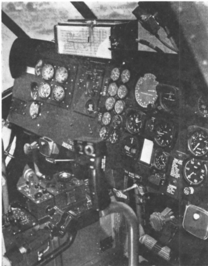
The Decca Equipment installed in the cockpit of the United States Army H 34 Helicopter
