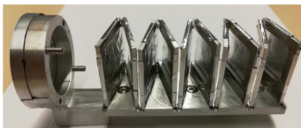
Figure 5. Lateral view of the detector with a longitudinal dimension of the base between the first and the last plate of approximately 90 \text{ mm} ( L_{10} = 90 \text{ mm} with L_0 = 0 ). The plates are separated from each other with a relative angle \phi = 12.5^\circ and have a dimension of L = 20 \text{ mm} .
