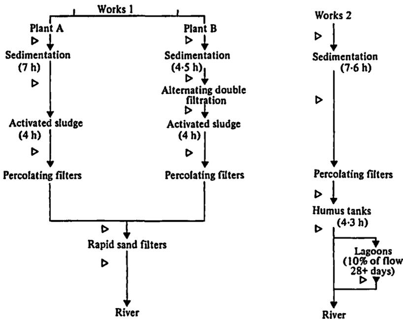
Fig. 1. Flow diagrams for the two wastewater treatment works. ▷, Sample points.
