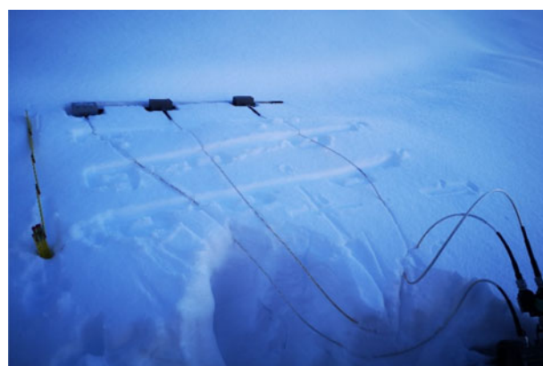
Fig. 8. Example of multiple placing of the radar at the top of the snowpack.
