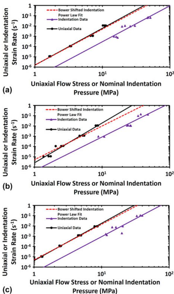
**Figure 4:** Plots of uniaxial [from 8] and nanoindentation steady state creep measurements in CsHSO<sub>4</sub> with power-law fitted curves and compared using the Bower shifted indentation power law fit. (a) 145 °C testing results, (b) 150 °C testing results, and (c) 160 °C testing results.
