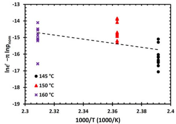
**Figure 3:** Temperature dependence of steady state indentation creep regime. As the indentation tests were conducted at CSRs, the Y axis is constructed to compare correlation between imposed test temperature and strain rate with measured output indentation pressure.
