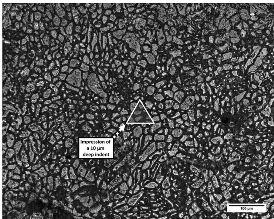
**Figure 8:** Micrograph of an etched CsHSO<sub>4</sub> specimen showing the grain structure of the test specimens. The translucent triangle at the center of the image shows the size of a Berkovich indenter imprint after being driven 10 μm into the surface. This image confirms that multiple grains are sampled during nanoindentation testing.
