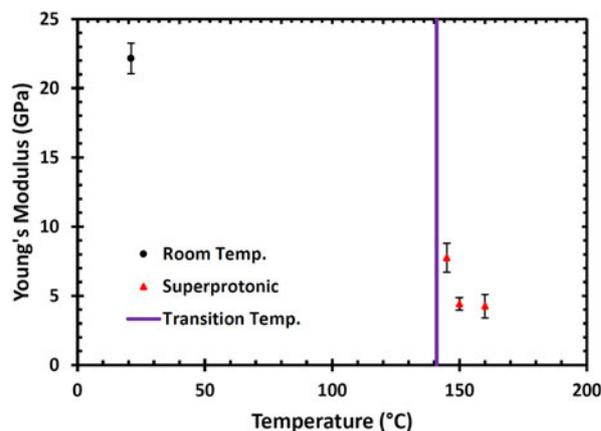
**Figure 5:** Average Young's modulus of CsHSO<sub>4</sub> as a function of temperature assuming a Poisson's ratio of 0.3. Error bars represent one standard deviation from the average modulus.
