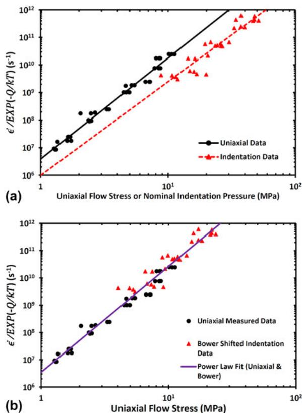
**Figure 6:** Comparison plot of uniaxial [from 8] and nanoindentation measured, temperature compensated power law creep in CsHSO<sub>4</sub>. (a) Indentation hardness compared with uniaxial flow stress. (b) Bower predicted flow stresses combined with true uniaxial measurements.
