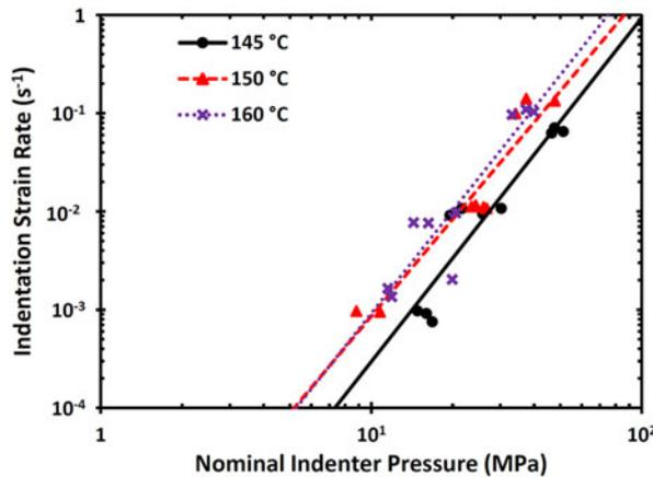
**Figure 2:** Nominal indenter pressures plotted as a function of imposed constant indentation strain rates at the 3 temperatures tested in the super-protonic phase; when fitted to a power-law function, a steady state creep deformation regime was attained during testing.
