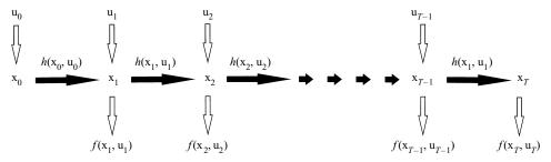
Fig. 1. Schematic presentation of a multiple-stage decision process over T stages with control variables  $(u_t)$ , state variables  $(x_t)$ , state equations  $(h(x_t, u_t))$  and stage output  $(f(x_t, u_t))$ . Maximization of a function of stage outputs over a planning horizon involves finding optimum control variables at each stage subject to the state equations at each stage and given the value of state variables at stage 0.
