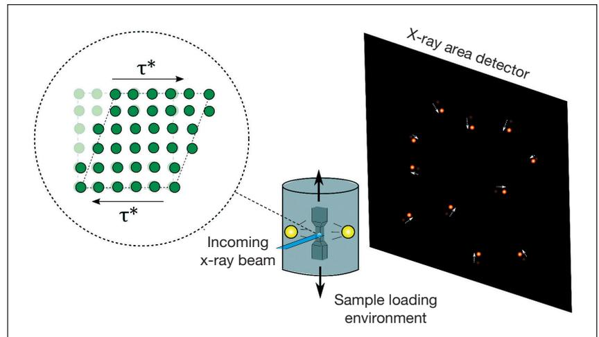
Using new high-energy x-ray techniques, deformation at the microscale can be probed deep within the bulk of deforming engineering alloys even in complex sample environments. From measured shifts in diffraction peak positions, the shear stresses ( $\tau^*$ ) required to permanently shift atomic planes relative to one another in individual deforming crystals comprising the samples can be deduced. Image Credit: Darren C. Pagan.
