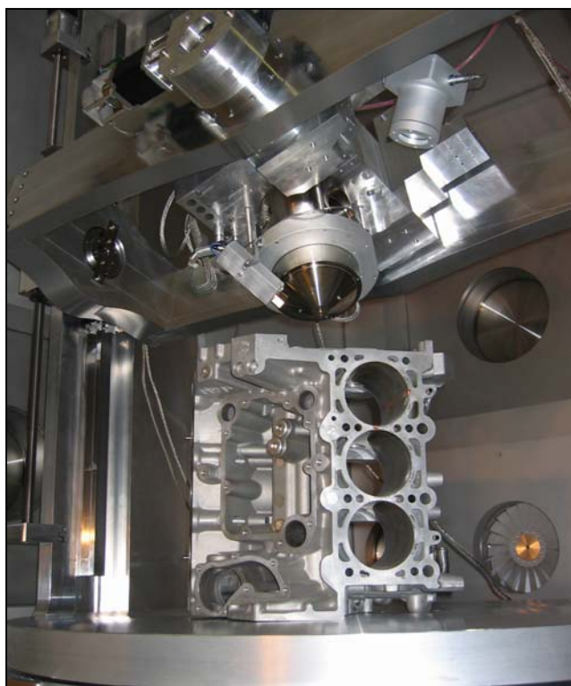
Fig. 2. A V-6 engine block in the LC-SEM with the column and backscatter detector positioned above.
