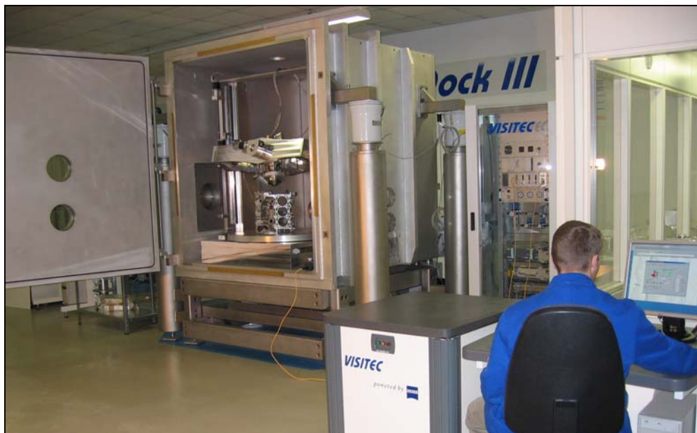
Fig. 1. The LC-SEM operator works at the control station while a V-6 engine block sits in the chamber ready to be examined.
