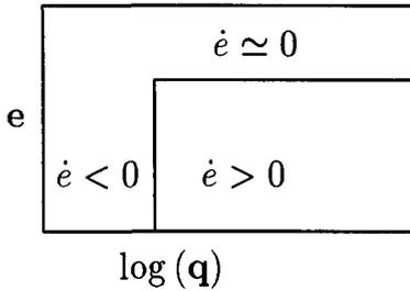
Figure 1. Regimes of  $\dot{e}$  in  $e - q$  plane (schematic only).
