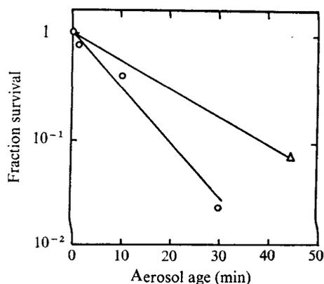
Fig. 4. Survival curves of phage  $\phi$ X174 aerosolized from 0.01% lysine at 74% r.h. in air containing 20–80 parts/ $10^9$  of ozone in the large system.
