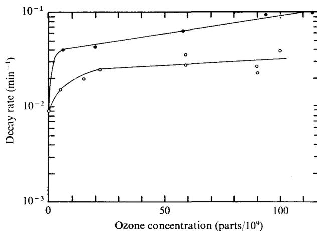
Fig. 2. Aerosol inactivation of phage  $\phi$ X174 as a function of the ozone concentration in the absence (○—○), and in the presence (●—●) of 500 parts/10<sup>9</sup> trans-2-butene at 96% r.h. (glass system, exposure time 30 min).
