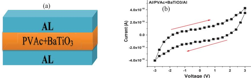
Fig.-5: (a) MIM structure. (b) Current–voltage behaviour of Al/PVAc + BTO/Al memory device.
