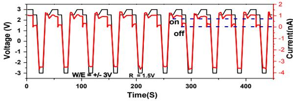
Fig-6: RWE characteristics of Al/PVAc+BaTiO<sub>3</sub>/Al device.
