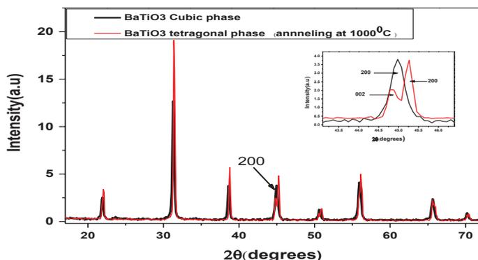
Fig-4: XRD patterns of BaTiO<sub>3</sub> nanoparticles as-purchased and BaTiO<sub>3</sub> nanoparticles annealed at 1000°C in the air. It can be observed the XRD data that the phase of nanoparticles has changed from cubic to tetragonal phase.
