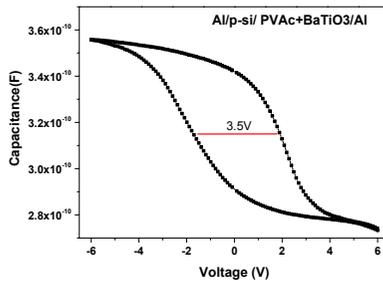
Fig.-7: C-V curves of MIS Structure (Al/p-Si/ PVAc+BaTiO<sub>3</sub>/Al).
